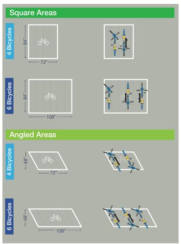
Note: Diagram reflects conceptual designs for bike hubs of two configurations and two sizes each. Hubs could also be sized to accommodate 8 or 10 bicycles where space allows and demand warrants. Some bike racks may be designated as hubs without painted areas, and some painted areas may not include bike racks.
