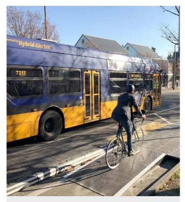
The new bus platform is installed on 108th Avenue NE, south of NE Second Street. It is made of 300 interlocking plastic panels that snap together, allowing for its rapid installation.
